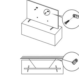
1. Using the appropriate screws, firmly fasten a set of brackets to the wall. Confirm that the screws are firmly attached to the wall.
